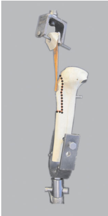
Figure 2. The biomechanical test setup used in the study. The dotted line indicates the osteotomy site.
