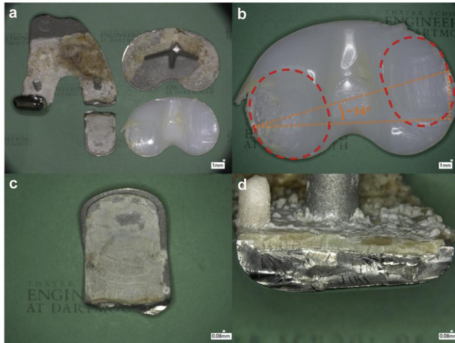
**Figure 5.** Biomechanical implant analysis. Explanted failed left Biomet Ascent TKA device including (a) a wide-angle image of all components, (b) damaged tibial polyethylene insert highlighting a significant adhesive/abrasive wear pattern (dashed) and  $\sim 14^\circ$  external femoral rotation (dotted), (c) fractured medial posterior condyle showing little cement adhesion, and (d) the fracture surface with beach marking throughout.
