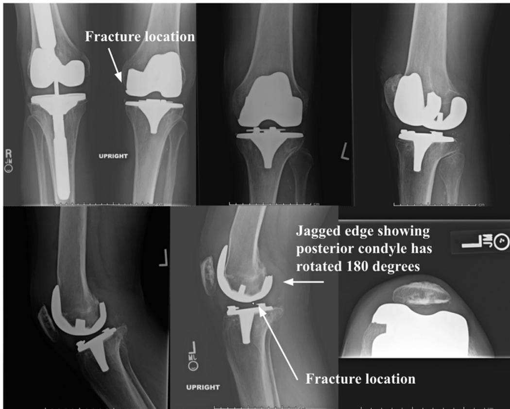
**Figure 3.** Radiographic left femoral component fracture. Multiple radiographs of the left knee demonstrating fracture of the femoral component after injury to the left knee 4 months ago. Arrows indicate fracture location on the anteroposterior view (top row, left) and lateral view (bottom row, middle). The lateral view (bottom row, middle) demonstrates that the posterior edge has rotated 180 degrees backward.
