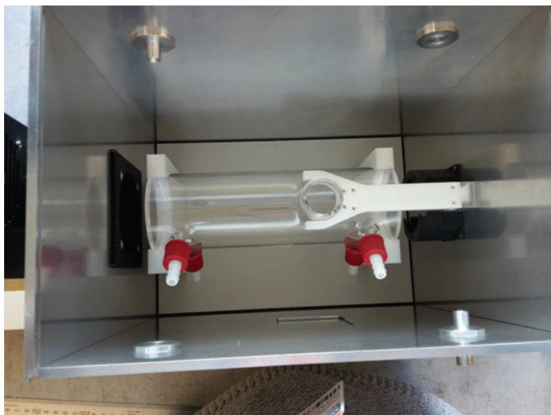
FIG. 2. Photograph of the quartz attenuator tube inside its mounting box. The Xe arc lamp is mounted to the left, outside of the box, the black interface plate can be seen to the left inside the mounting box. The sample is loaded through the circular opening in the top of the tube so that it is positioned at the focus of the Xe lamp. Color images are available online.
