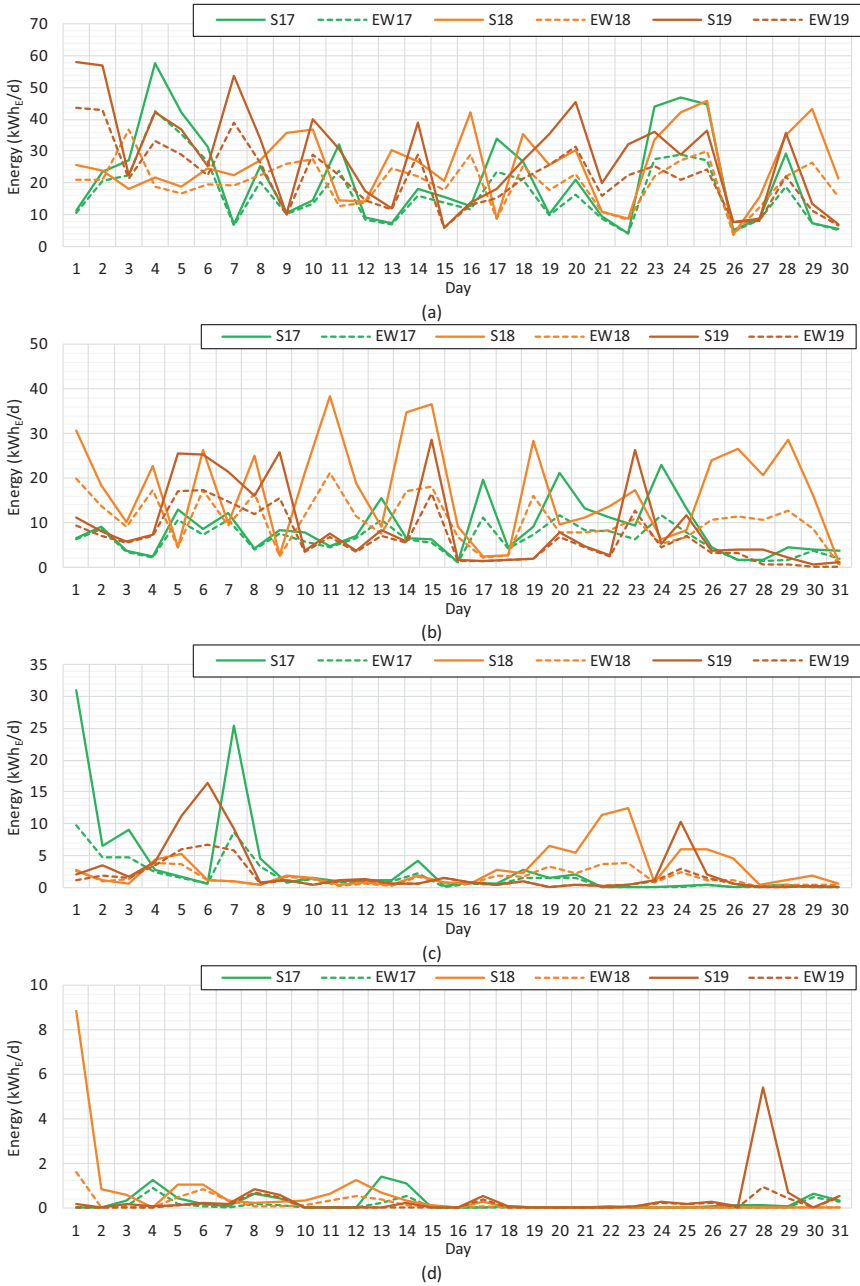
Fig. 5. Solar PV electricity at the daily level during the period of 2017–2019. (a) September. (b) October. (c) November. (d) December.
