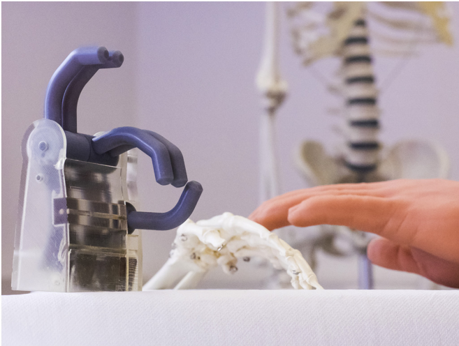
Fig. 1. 3D-printed polymer replica of the first, artificial “iron hand” of Götz von Berlichingen (see left side) based on the work in [8]. The replica was printed from computer-aided design (CAD) data by a 3D multi-material printer, Stratasys J750, that allows for the production of transparent components, offering insights into the mechanics of the hand. Picture credits: Offenburg University, Germany.
