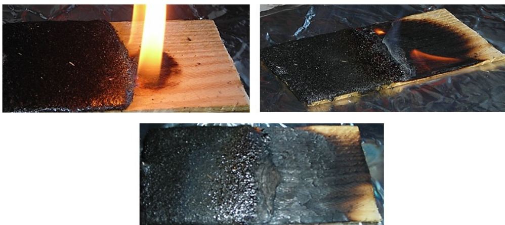
Figure 8. Flame propagation over the surface of a sample with a flame-resistant coating applied only to a part of its surface.
