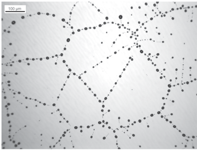
Fig. 1. Stationary droplet patterns emerging from a uniform PS(10.3k) film of thickness h_\infty = 110 nm after dewetting at T = 120^\circ\text{C} from a hydrophobically coated Si wafer: (Left) AF1600 coating and (Right) DTS coating (21).
