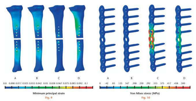
The predicted minimum principal strains within the bone using screw configuration C1234 at a load of 500N. The letters A to D correspond with the loading conditions considered in this study.
