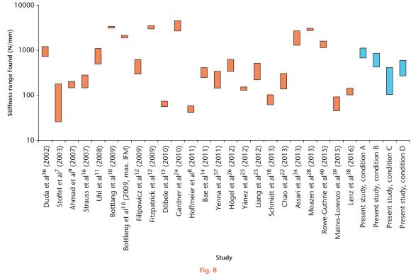
The recorded stiffness values of locking plate constructs found by previous studies (orange bars) and the stiffness values of each of the loading conditions used in this study (blue bars). IFM, interfragmentary motion.
