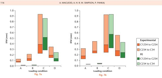
The mean experimentally measured axial interfragmentary motion (IFM) and predictions using the finite element (FE) simulation for each loading condition and screw configuration considered in the study for a) the narrow locking plate using a load of 100N, and b) the broad locking plate using a load of 200N.
