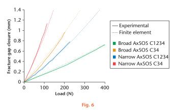
The load-displacement plots for the experimental and finite element cases using loading condition C. Results are shown for the two plate types (Stryker AxSOS broad and narrow plates), and for the shortest and longest working lengths evaluated in the study.
