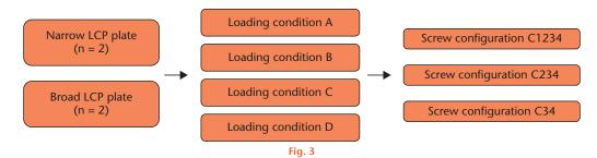
The testing regime used for the composite tibia specimens. Two locking compression plate (LCP) types, four loading conditions, and three screw configurations were evaluated.
