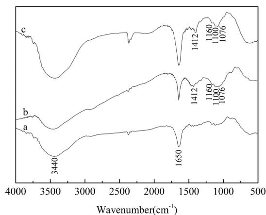
**Figure 1.** FTIR spectra of Xuan papers: (a) untreated, (b) X-AP4, and (c) X-AP10.
