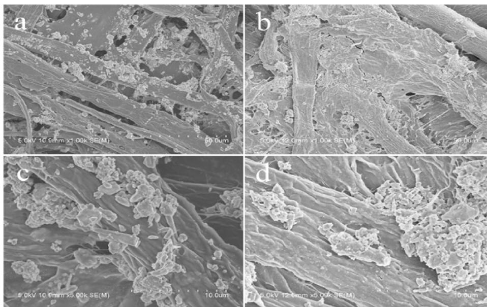
Figure 7. Morphology of the char residues of treated Xuan paper after VFT at low magnification (×1000): (a) X-AP6, (b) X-AP10 and high magnification (×5000): (c) X-AP6, (d) X-AP10.
