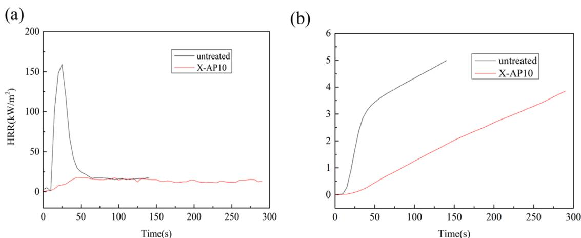
**Figure 4.** Heat release rate (a) and total heat release curves (b) of untreated and flame-retardant-treated Xuan papers.
