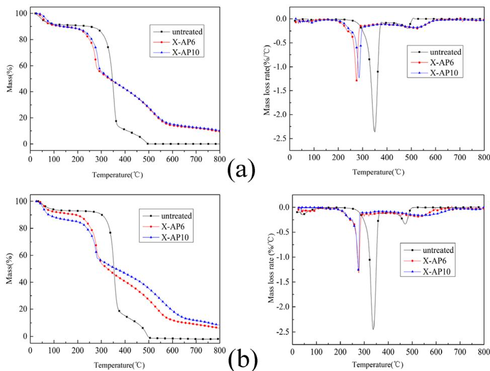
**Figure 5.** TG and DTG curves of untreated and treated Xuan papers under (a) nitrogen and (b) air atmosphere.
