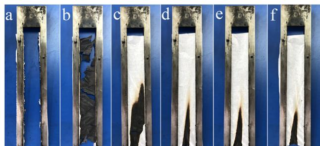
**Figure 3.** Digital images of Xuan papers after VFT: (a) untreated, (b) X-AP2, (c) X-AP4, (d) X-AP6, (e) X-AP8, and (f) X-AP10.
