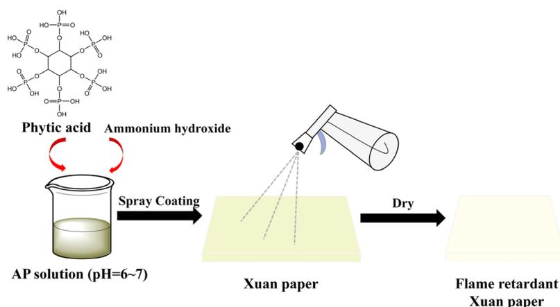
Figure 11. Schematic representation of spray coating of Xuan paper.
