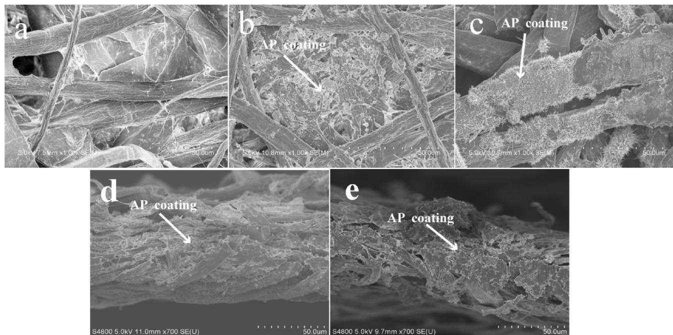
**Figure 2.** Surface morphologies of Xuan papers: (a) untreated, (b) X-AP6, (c) X-AP10, and cross sections of (d) X-AP6 and (e) X-AP10.
