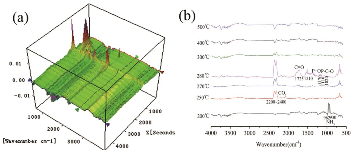
Figure 6. Three-dimensional diagram (a) and FTIR spectra (b) of volatiles of treated Xuan paper (X-AP10) at different temperatures.
