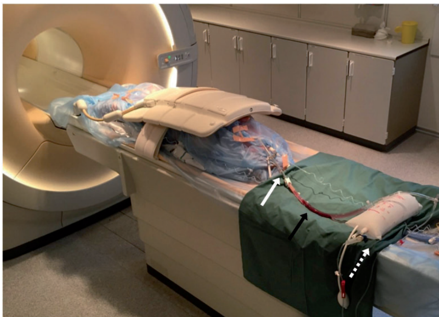
Fig. 3. Experimental set-up. A pig is lying on the flat bed in the MRI scanner. It is wrapped in plastic to avoid risk of contaminating the scanner. On top of the pig is the coil. On the green cloth is the tube with the PE suspended in saline (black arrow). Attached are the cannula with a plastic clamp (white arrow) and the MRI-safe pressure bag (dashed white arrow).
