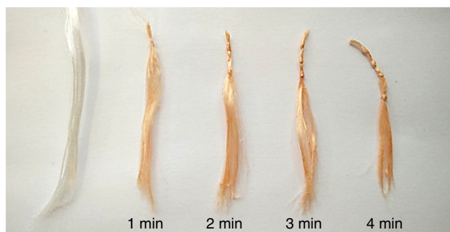
Fig. 7 Optimization of the plasma treatment time for UHMW-PE fibrous material with DR1-A. Each picture of the treated fibrous material after purification is taken compared to an untreated reference sample of the used material
