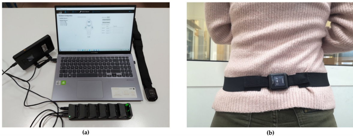
Figure 1. (a) Opal System: Access Point, Docking Station, Opal Sensor and Mobility Lab software. (b) Placement of the Opal Sensor in lumbosacral region through an elastic belt.
