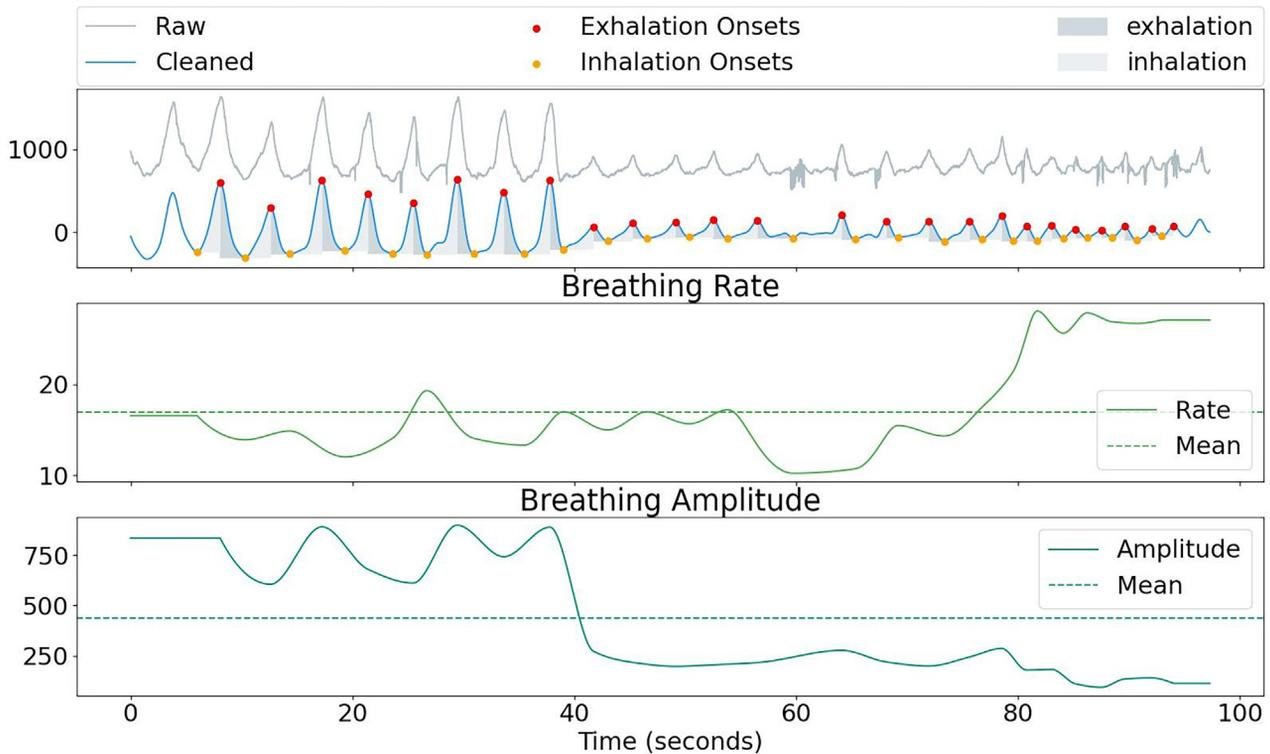
**Figure 4. Raw data, filtered data, breathing rate, and breathing amplitude of the data collected from the belt during standing**
