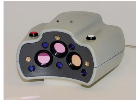
FIGURE 4: The hand-held imaging unit is about 6 inches wide and 8 inches deep. The white button activates the blue lights and red lasers, both of which are blocked by the green bandpass filter and are not imaged. The red button is for recording.
