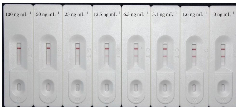
FIGURE 4: CGIC strips showing color changes corresponding to the concentrations of aloë-emodin. The cutoff value for aloë-emodin was 50 ng mL -1 .
