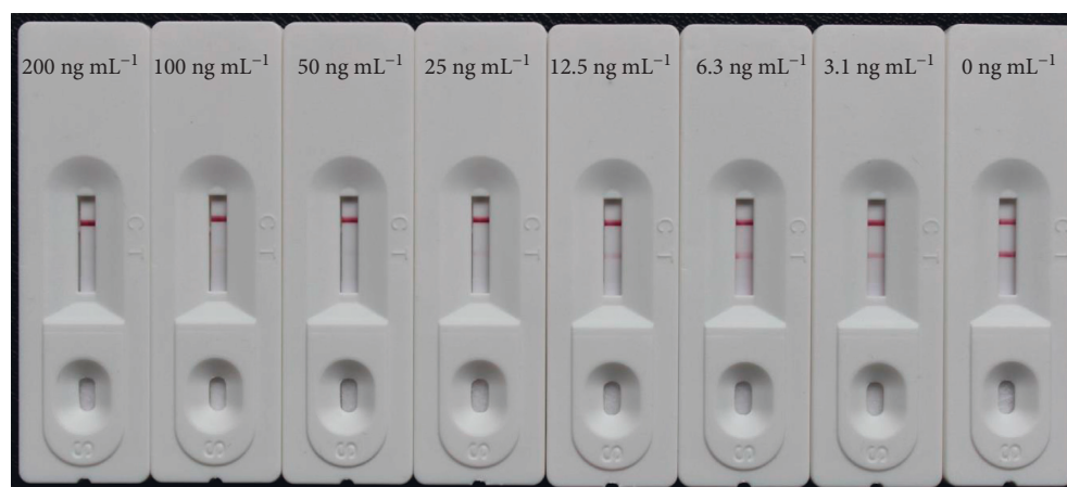
FIGURE 3: CGIC strips showing color changes corresponding to the concentrations of rhein. The cutoff value for rhein was 50 \text{ ng mL}^{-1} .
