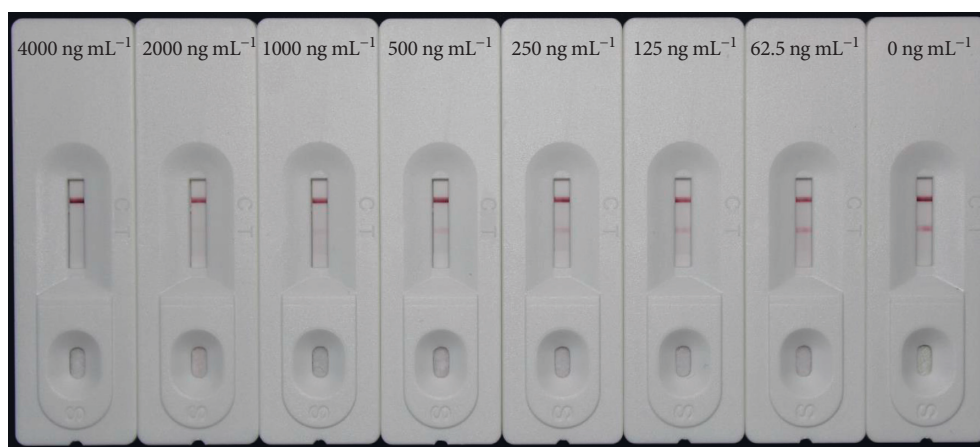
FIGURE 5: CGIC strips showing color changes corresponding to the concentrations of emodin. The cutoff value for emodin was 2000 ng mL -1 .
