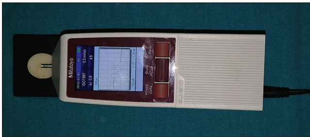
Figure 2: Surface roughness analysis of prepared samples
