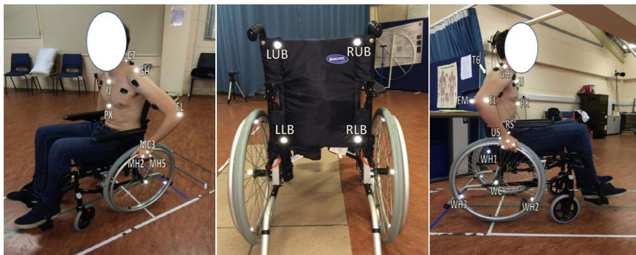
Figure 2. Markers set placement on the trunk, right upper limb and the wheelchair.
