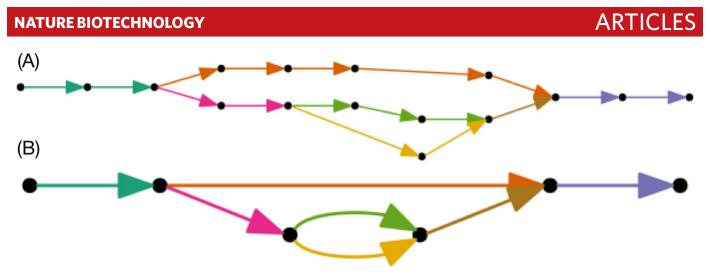
**Extended Data Fig. 5 | Assembly Graph. (A)** A marker graph with linear sequence of edges colored. **(B)** The corresponding assembly graph. Colors were chosen to indicate the correspondence to marker graph edges.
