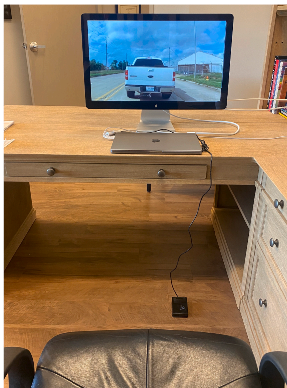
Fig. 1. Subjects watched a simulated driving video on a large screen with a mock brake pedal.
