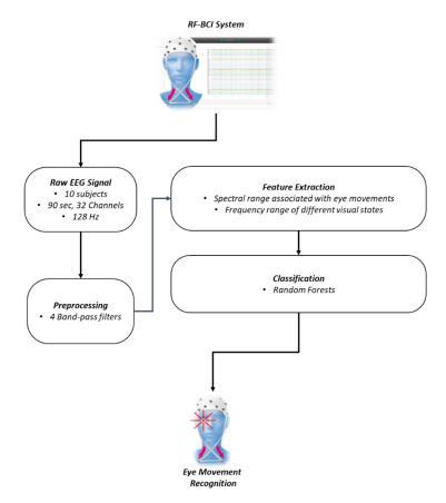
**Figure 1.** The random forests brain–computer interface (RF-BCI) system architecture. Initially, the EEG signal is captured using the headset and undergoes a preprocessing filtering procedure for removing the unwanted noise and separate the bands. The next step is the feature extraction and the association of each dataset entry with an eye movement. Finally, the dataset is used to train the RF classifier.
