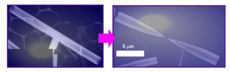
**Figure 7.** Fullerene micro-horns can be fabricated from fullerene micro-tubes of  $C_{60}$  and  $C_{70}$  mixture (these images are representative ones).
