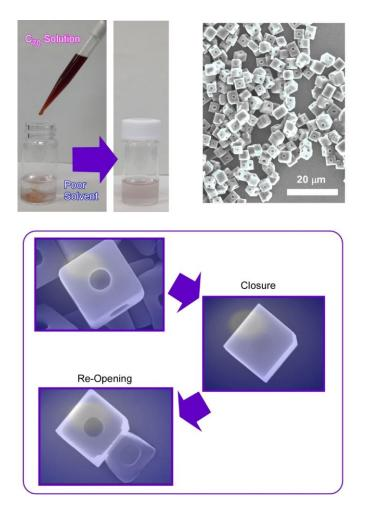
**Figure 5.** C<sub>70</sub> holes-in-cube structure with one regular micro-hole at the center of every face in the cubic structures and its shape-shifts for closure and re-opening of the micro-hole.
