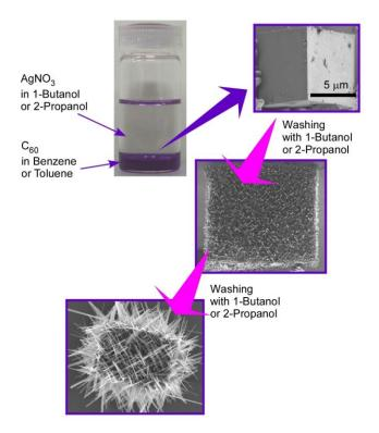
**Figure 3.** Hierarchic rods-on-cube structures of  $C_{60}$  assembly fabricated through shape-shifting from micro-cube structures prepared with  $C_{60}$  and AgNO<sub>3</sub> via the LLIP method.
