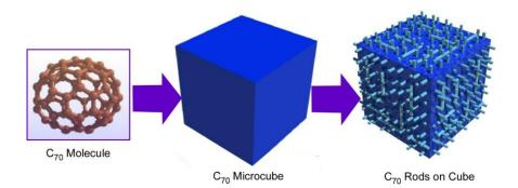
**Figure 4.** Hierarchic rods-on-cube structures of  $C_{60}$  assembly fabricated through shape-shifting from micro-cube structures prepared with  $C_{70}$  molecules.
