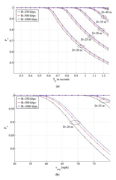
**Figure 4.** Illustrating  $P_{success}$  for various data rates *R* and coverage distances *D*. (**a**) Varying beacon interval with  $v_{avg} = 70$  mph, (**b**) Varying average vehicle speed with  $T_b = 0.7$  s.
