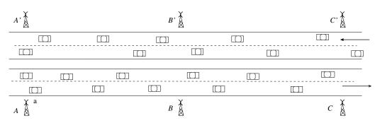
Figure 1. Illustrating a highway segment with several TMUs [85] ©IEEE.
