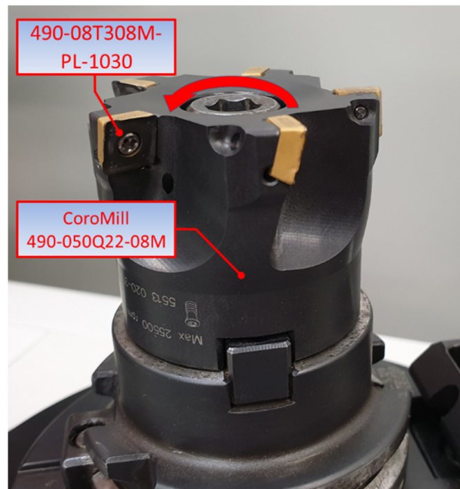
Figure 2. View of the CoroMill 490-050Q22-08M head by Sandvik Coromant.
