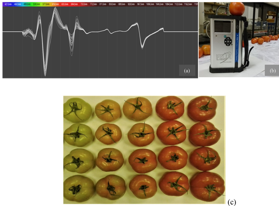
Fig 1. Raw spectra curves of all tomato samples at various stages of fruit maturity (a), NIR measurements of tomatoes (b), and the five stages of fruit maturity in vertical rows (c): Vertical rows from left to right; (1) Breaker, (2) Turning, (3) Pink, (4) Light-red, (5) Red. Fresh tomato fruits were labeled and scanned using the handheld near infra-red enhanced spectrometer (F-750, Produce Quality Mater, Felix Instruments, Camas WA, USA), at wavelength range (285–1200 nm).
