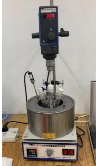
Figure 1. Preparation device for the MMA repair material.
