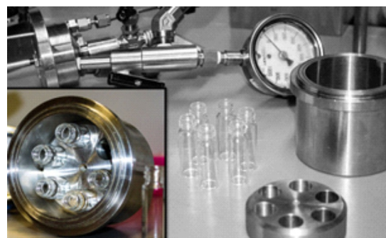
Figure 2. Parallelized hydrogenation setup in Parr TM pressure reactors.
