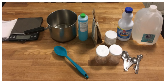
FIG. 1. Simple supplies used for phantom construction. Dilute bleach was used to sterilize the surfaces of all components prior to fabrication, and a solution of agar-agar powder, distilled water, and copper sulfate were used for the gel.
