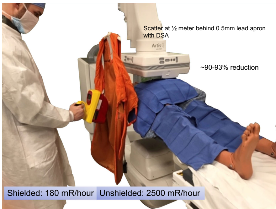
FIG. 17. The protection afforded by the lead apron personal protective equipment (PPE) is quickly made, and questions arise as to options with specified lead equivalence and weight/benefit advisement.
