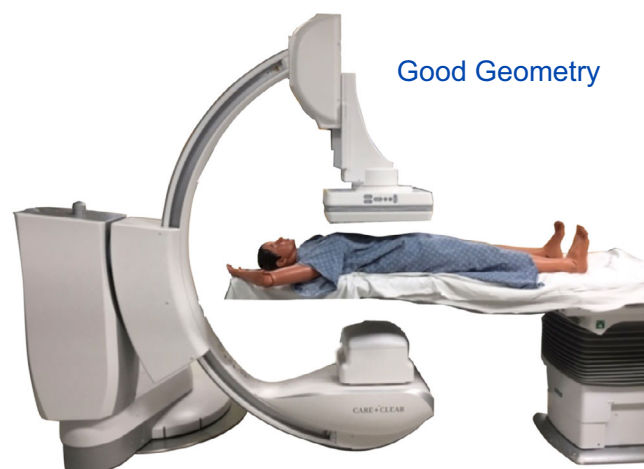
FIG. 4. The concept of isocenter and the need to angle the C-arm about a vessel is given, noting that the isocenter to focus is fixed while the image receptor allows movement. Having the vessel of interest at isocenter allows the image to remain in the image with C-arm angulations.
