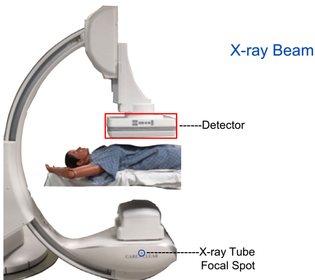
FIG. 2. The class is joined together in visual inspection of a “dot” or marking on the tube housing which depicts the focus and the origin of x rays, the low absorbing table and pad, and the image receptor.
