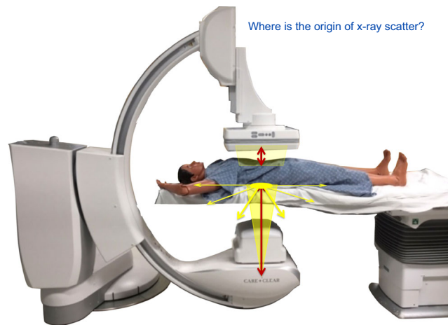
FIG. 3. The origin of scatter is stated to be the area of the back of the supine patient struck by the x-ray beam. The example of a flashlight beam striking the instructors hand causing large amounts of scattered light has been used as a visual.
