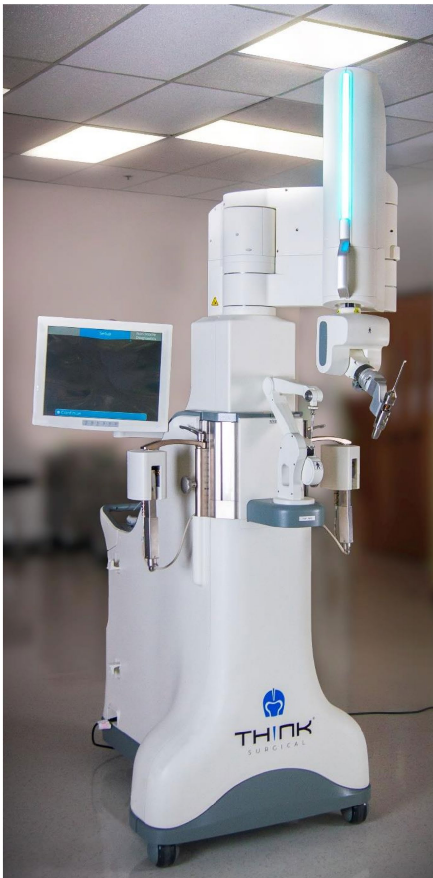
Fig. 1 Robotic-assisted surgery device (310 TCAT®, TSOLUTION ONE® Total Knee Application, Think Surgical Inc., Fremont, CA, USA)
