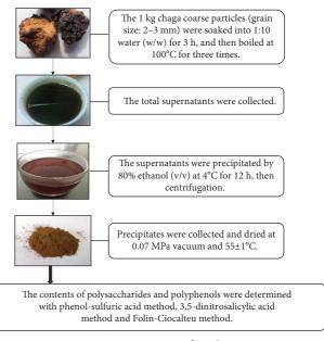
FIGURE 3: Extraction flowchart.
