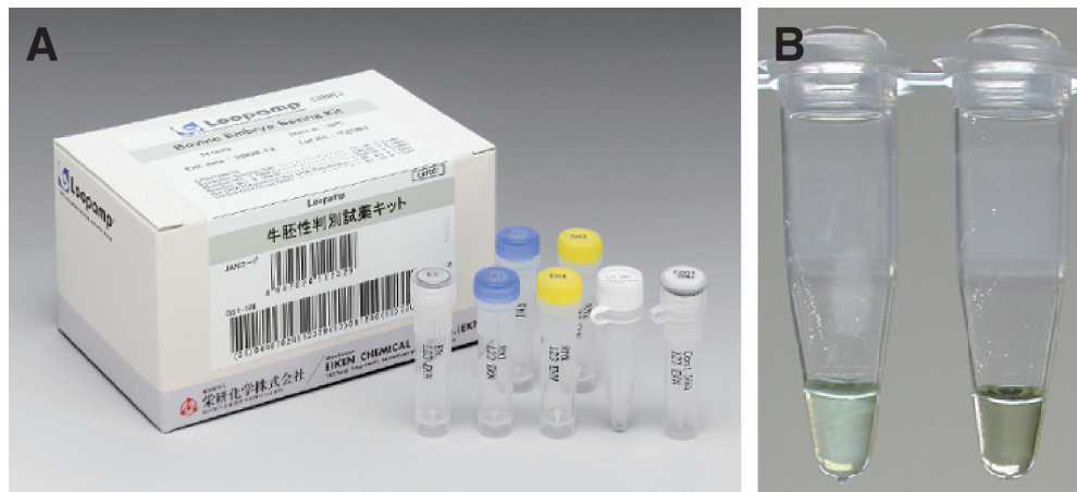
Fig. 2. Bovine embryo sexing kit with LAMP (A) and detection of DNA amplification by the turbidity of reaction mixture (B). The reaction tube on the left side in panel B shows the white precipitate of magnesium pyrophosphate yielded by LAMP reaction.
