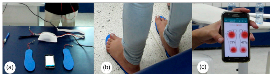
Figure 1. Components of the prototype baropodometric insole. A Baropodometric insole prototype. B Static position to determine the limit of symmetry between the affected and unaffected hemibody. C Mobile health application developed to diagnosis and monitoring weight-bearing asymmetry.
