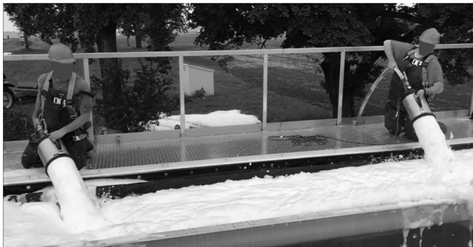
FIGURE 3 View of the modified rendering trailer canopy during filling of medium-expansion water-based foam. Safety harnesses were attached to the railing and protective gear was worn by the staff members. Third staff member and nozzle used in the trial is not in view.
