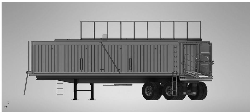
FIGURE 2 Schematic of a 64.5-m 3 (dimensions 12.2 × 2.36 × 2.24 m; length, width and height) modified rendering trailer used in Trial 2. Customizations included a top-hinged side to side half width/whole gate with attached loading ramp, and mid-length for added compartmentalization, safety railings on top, hard-top half-width steel reinforced canopy and a hydraulic lift system. Schematic, courtesy of Brown Industrial, Inc.
