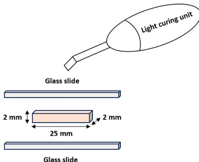
Fig. A. Schematic presentation of specimen preparation for flexural strength and elastic modulus tests.
