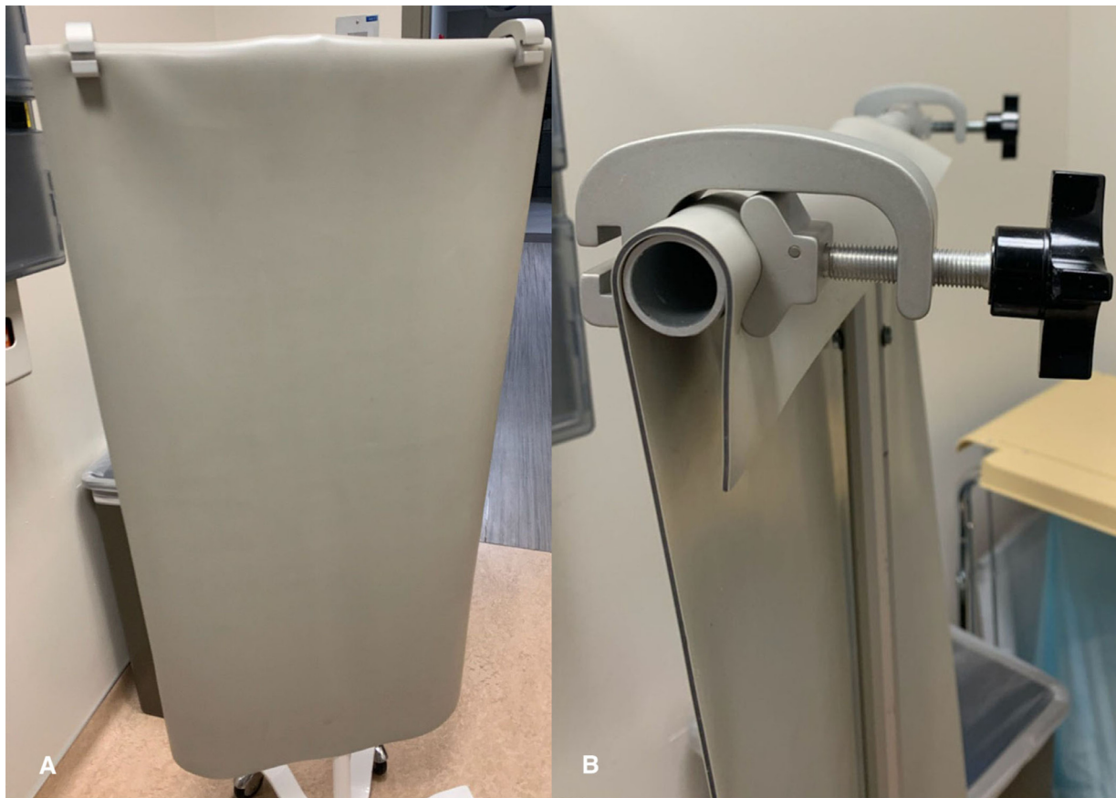
FIG. 3. Protective lead shield. (A) Improvised shield for protecting nursing staff in the room. The vinyl lead sheet is easy to clean and the structure is lightweight. (B) Close-up of clamps used to affix lead sheet to frame. (Color version of figure is available online.)
