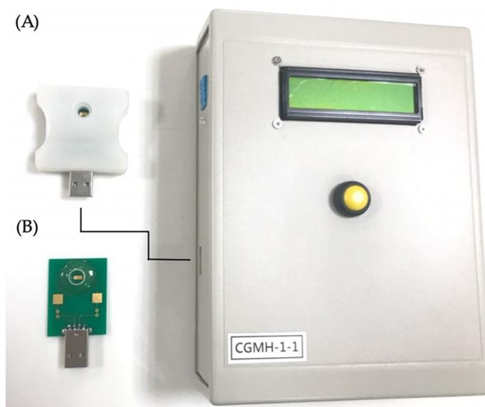
**Figure 1.** Measuring of salivary conductivity with the portable biodevice. (A) Salivary samples were applied to the well of the sensing probe. The sensing probe was connected to the conductivity meter through a USB port and read out the data immediately after pressing the yellow button. (B) The disposable printed-circuit board (PCB) of the sensing probe inside the shelter and the electrode were placed in horizontally parallel.
