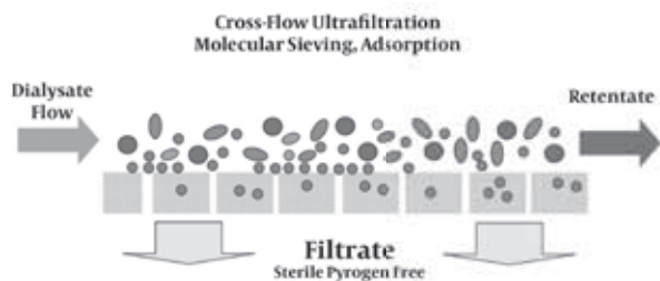
Figure 1. Cold Sterilization Process Based on Ultrafiltration
