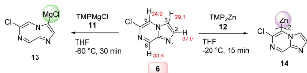
Scheme 4 Thermodynamically driven regioselectivity switch in the metalation of 6-chloroimidazo[1,2- a ]pyrazine using either \text{TMPMgCl}\cdot\text{LiCl} ( 11 ) or \text{TMP}_2\text{Zn}\cdot 2\text{MgCl}_2\cdot 2\text{LiCl} ( 12 ). Salts are omitted for clarity.
