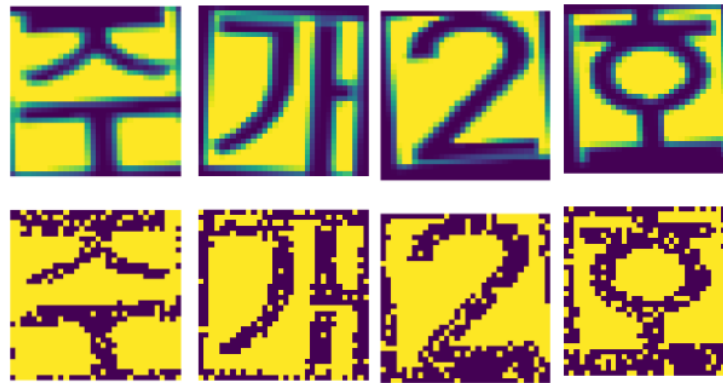
Figure 5. Images from the License plate dataset are converted into spikes using Poisson distribution. The upper images show original images, and the below images represent the spike version of original images.
