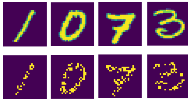
Figure 7. Original images of the MNIST dataset are converted into spikes using Poisson distribution. The upper images show original images, and the below images represent the spike version of original images.
