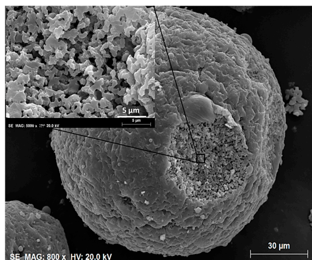
Figure 27. Macro/mesoporous epoxy-functionalized silica microspheres (MICROSCAFS), synthesized from TEOS and GPTMS, obtained by emulsion combined with sol-gel transition and phase separation, in the absence of any gelation or phase separation inducer additive. Reprinted from Microporous Mesoporous Mater. , Vol. 261, M.V. Loureiro, M. Vale, A. De Schrijver, J.C. Bordado, E. Silva, A.C. Marques, Hybrid custom-tailored sol-gel derived microsc scaffold for biocides immobilization, Pages 252–258, Copyright (2018), with permission from Elsevier [140].
