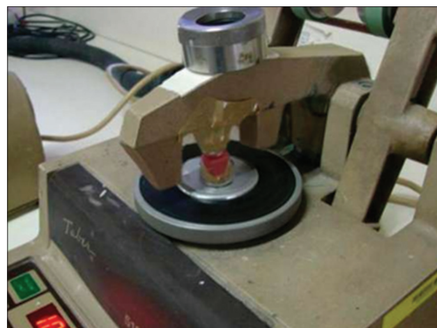
Figure 12: Samples mounted against each other on a wear machine during testing
