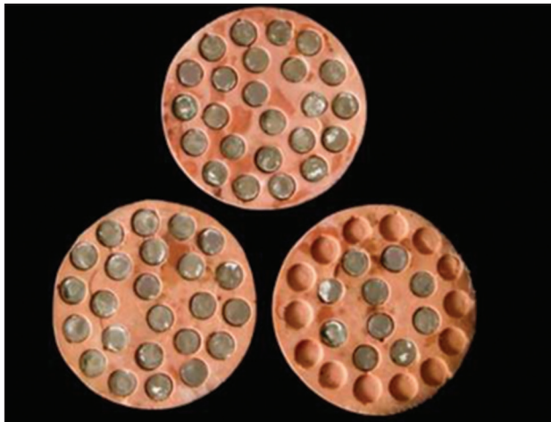
Figure 3: Metal discs secured in refractory casts
