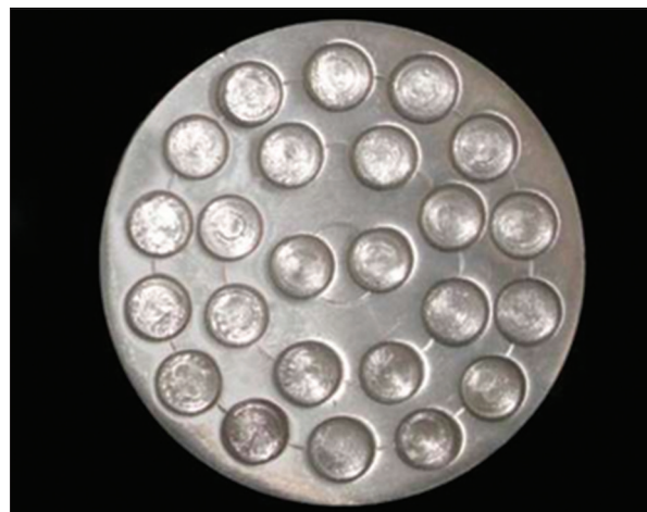
Figure 1: Custom milled steel template with standardized moulds
