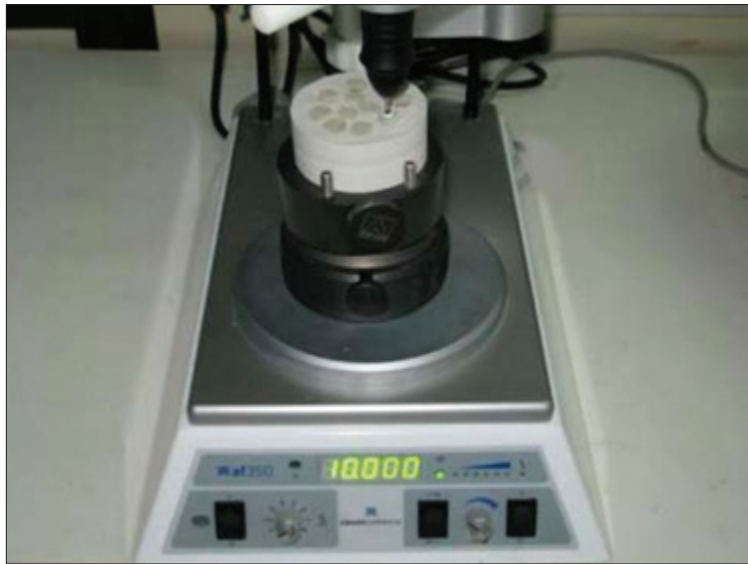
Figure 5: Discs stabilized on the milling machine to simulate chair side adjustments
