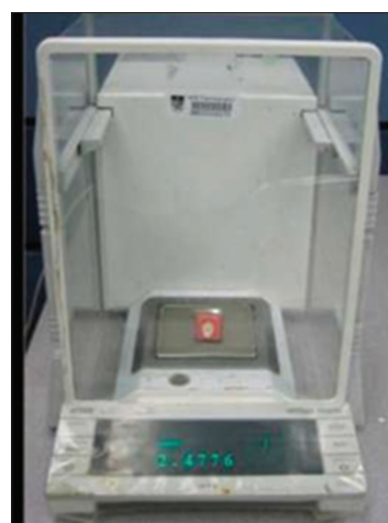
Figure 11: Electronic analytical balance of 0.0001g accuracy
