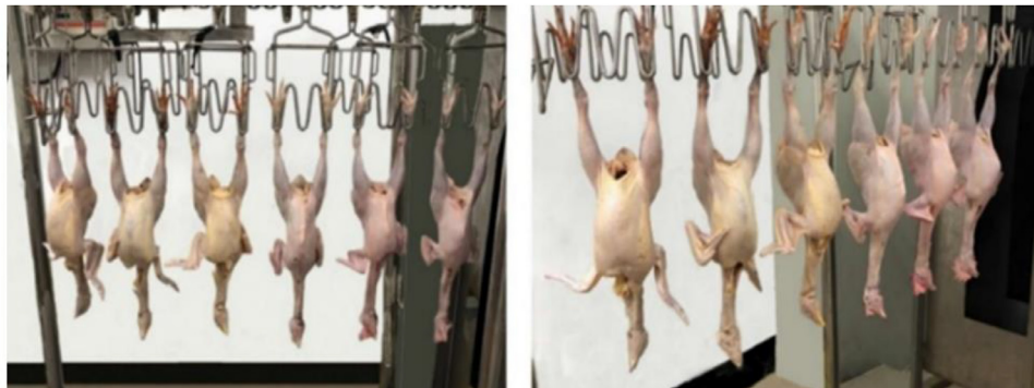
Figure 2. Chicken carcasses positioned on an online processing conveyor system for automated volume estimation (A) Frontal view showing the orientation and spacing optimized for 3-D imaging (B) Side view illustrating a different camera angle.
