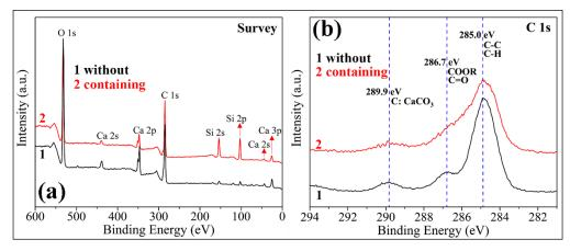
**Figure 8.** XPS spectra of two kinds of PC coatings (without using hydrophobic emulsion and containing hydrophobic emulsion): (**a**) survey spectra; (**b**) high resolution spectra in C 1s region.
