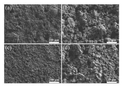
**Figure 7.** FE-SEM images of two kinds of PC coatings: (**a**) and (**b**) PC coatings without using hydrophobic emulsion; (**c**) and (**d**) PC coating containing hydrophobic emulsion.
