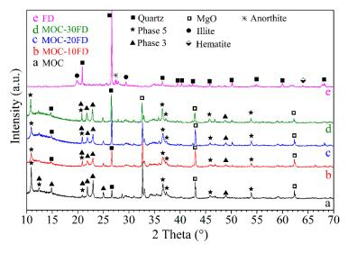
**Figure 2.** XRD patterns of different samples: a. pure MOC; b. FD/MOC composites containing 10 wt.% of FD; c. FD/MOC composites containing 20 wt.% of FD; d. FD/MOC composites containing 30 wt.% of FD; e. FD powders.
