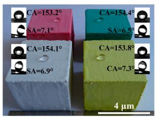
**Figure 6.** Superhydrophobic PC coatings with various colors, the substrates used are FC/MOC composites containing 30 wt.% FD.
