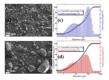
**Figure 1.** (a) SEM image of MgO particles; (b) SEM image of FD particles; (c) particle size distribution of MgO powder; (d) particle size distribution of FD powder.
