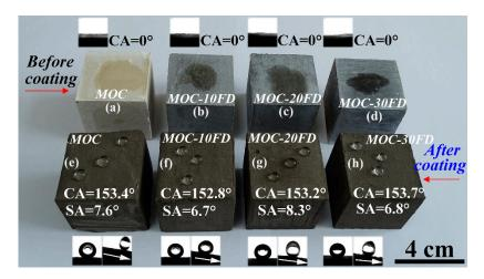
**Figure 5.** Photograph of the wetting behavior of water droplets on various FD/MOC composite surfaces. (a)–(d) before coating treatment; (e)–(h) after coating treatment. The inset show the CA and/or SA measurement.
