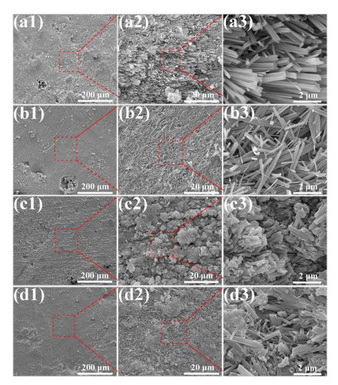
**Figure 4.** SEM morphologies of the as-prepared surfaces of different samples. (**a1**), (**a2**) and (**a3**) pure MOC; (**b1**), (**b2**) and (**b3**) MOC-10FD; (**c1**), (**c2**) and (**c3**) MOC-20FD; (**d1**), (**d2**) and (**d3**) MOC-30FD.
