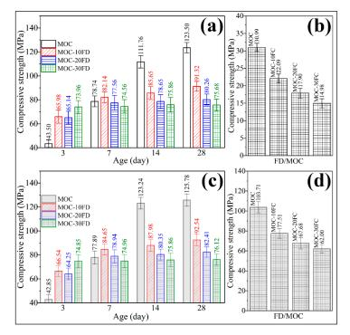
**Figure 9.** Compressive strength measurement of the FD/MOC composites. (a) FD/MOC composites without coating before soaking in water; (b) FD/MOC composites without coating after soaking in water; (c) FD/MOC composites containing coating before soaking in water; (d) FD/MOC composites containing coating after soaking in water.
