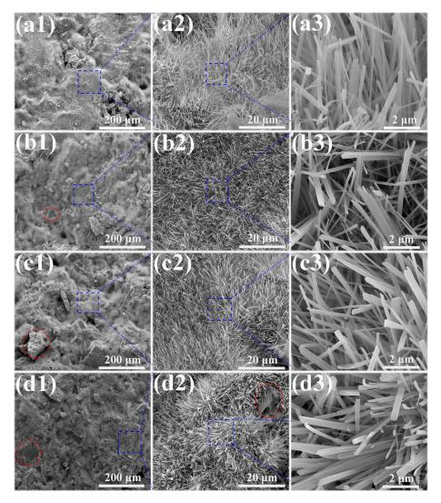
**Figure 3.** SEM morphologies of the fractured surfaces of different samples. (**a1**), (**a2**) and (**a3**) pure MOC; (**b1**), (**b2**) and (**b3**) MOC-10FD; (**c1**), (**c2**) and (**c3**) MOC-20FD; (**d1**), (**d2**) and (**d3**) MOC-30FD.
