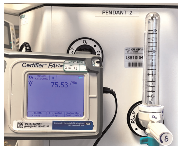
Figure 1 An example of the measured flow rate when a flowmeter is fully opened.
