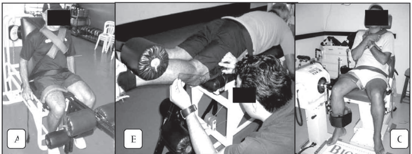
Figure 2 – (A) Positioning of the volunteers in the modified isometric dynamometer (MID) to collect isometric extension torque data. (B) Positioning of volunteers in the MID to collect isometric flexion torque data. (C) Positioning of volunteers in the Biodex System 3 to collect the flexor and extensor isometric and isokinetic torque data.
