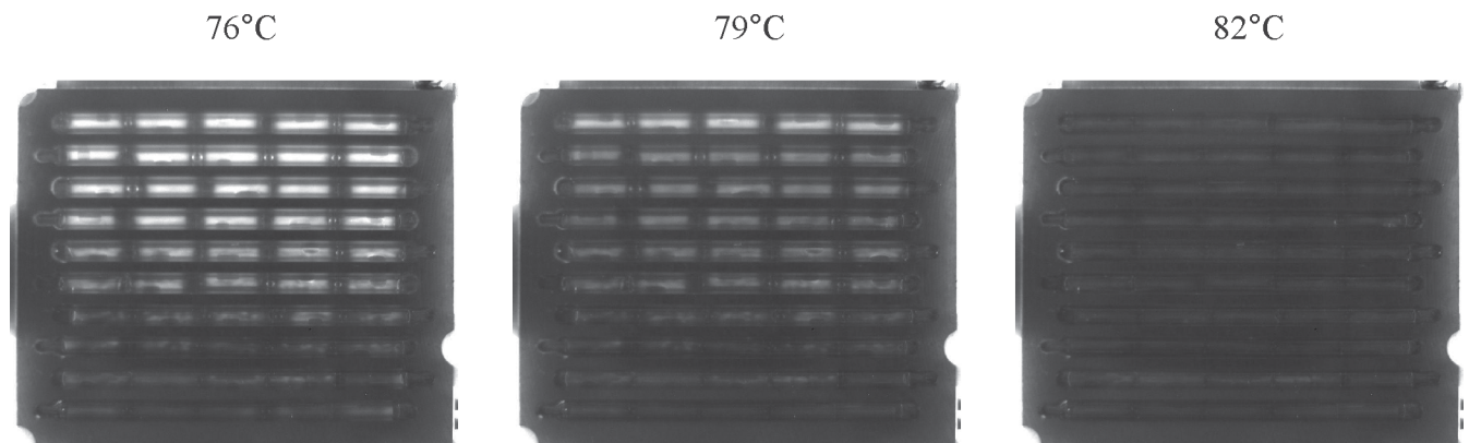
Fig 9. Photographs of the cassette during melt curve data collection. These images were taken during the MCA after 35 cycle PCR with stx2 primers. The corresponding melt peaks are shown in Fig 12.
