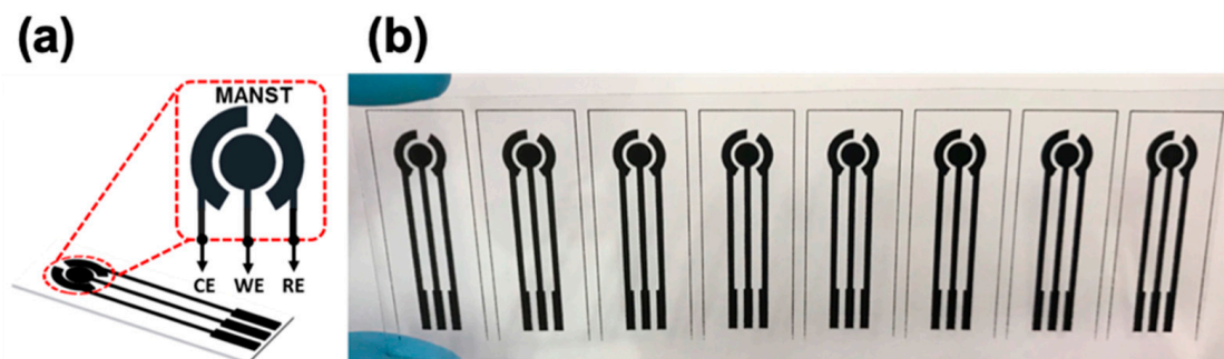
Figure 1. (a) Schematic of the carbon-based three-electrode system showing the working (WE), counter (CE), and reference (RE) electrodes. (b) Photographic image of an obtained batch of screen-printed carbon electrodes (SPCEs) on a flexible PET substrate.
