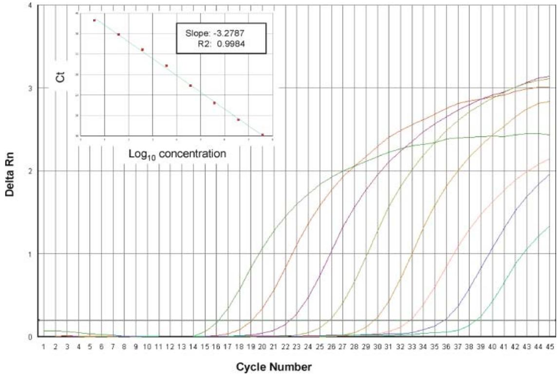
Fig. 3. Dynamic range of hAdV detection. Amplification curves (Delta Rn vs. Cycle) and standard curve (Ct vs. log<sub>10</sub> concentration) for serial dilutions of the hAdV4 plasmid showing the assay dynamic range ( $3.8 \times 10^0$  copies/reaction to  $3.8 \times 10^7$  copies/reaction).
