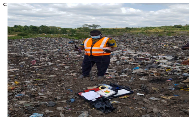
Fig. 2(c). Measurement of pH, EC, TDS and temperature at urban dumpsite.
