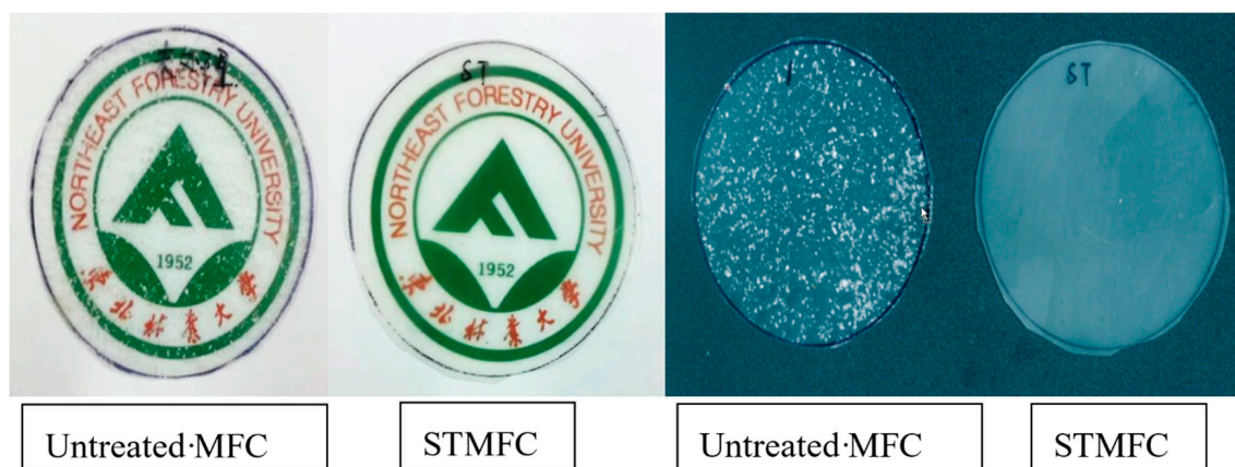
Figure 5. Scanning images of LLDPE composite films enhanced by 10 wt% MFC with different processing methods.
